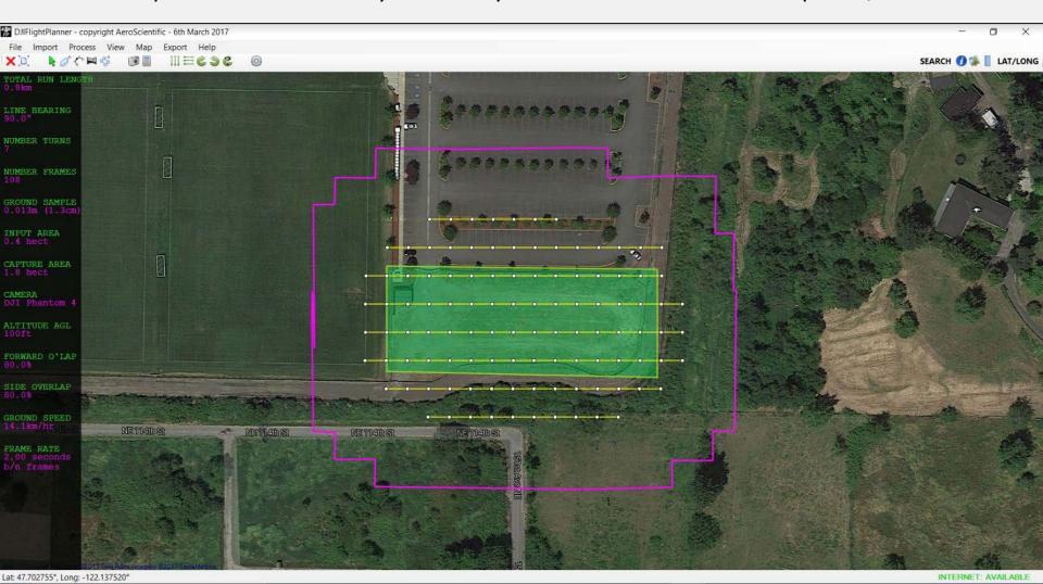
• After tidying up the plan by deleting any unwanted points/lines, observe the left-hand-side of the screen which shows various parameters for your planned flight path. In this example, the flight path requires three "turns" with a quantity 52 frames to be captured. The ground sample distance (GSD), or 'pixel size', will be approx. 1.3cm. The next slide illustrates how you can export the flight plan in .csv format for use in Litchi.
