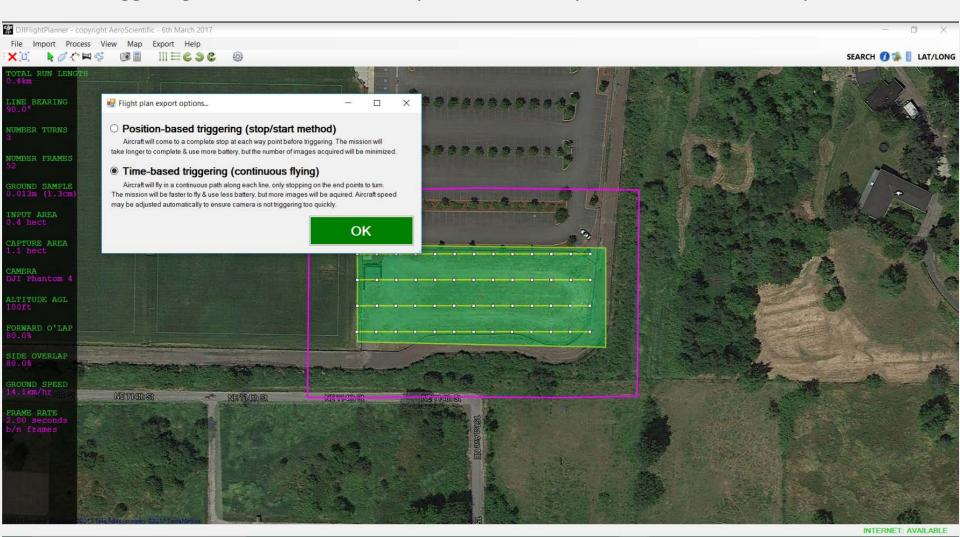
• **IMPORTANT** - if you choose 'time-based' triggering, the drone will fly continuously through the entire flight plan without stopping. This makes flight plans much quicker to fly and saves battery. It will trigger the camera based on time to achieve the desired forward overlap. A message like the following will appear, reminding you to take note of the 'cruising speed' and 'frame-rate', as you will need to enter these parameters in Litchi.
