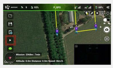
• When the drone reaches the first way point (start of the first flight line), it will pause for 10 seconds. During this time, start the camera triggering by pressing the "TL" button. When the mission has finished, the drone will fly home & land automatically if you have the "Finish Action" set to "Go Home", or you can press the green & white "Return to Home" button to land the aircraft.
