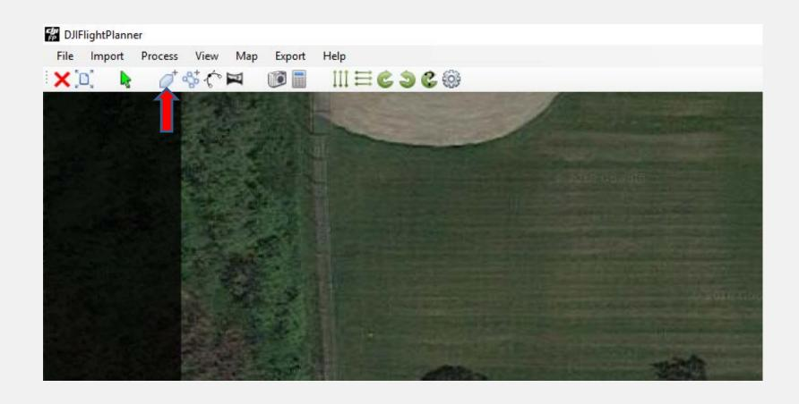
Once your area has been marked, press ENTER or ESCAPE to close the polygon. The "Camera, imaging & miscellaneous parameters..." dialog box will be presented. There are several parameters that can be entered, but for this small example, simply choose your drone from the drop-down list of choices, and revise **Altitude** to 100 feet. Then press the green "ACCEPT" button.
